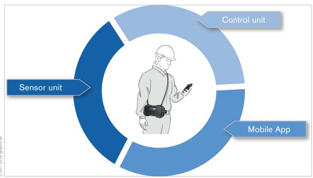
The Dräger X-pid® 9500/ X-pid 9500+ consists of three elements: You control the sensor unit via the control unit and the preinstalled mobile app. The sensor unit can be worn around the neck, keeping one hand free.
