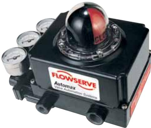
The Automax Apex 8000 positioner provides outstanding control for a wide range of valves and dampers. The two-stage pneumatic relay provides fast, sensitive response characteristics to meet demanding control objectives. It may be used with 3-15 psi pneumatic control signals or fitted with an I/P transducer for 4-20 mA signals. The Apex 8000 is available with many options including position feedback limit switches, 4-20 mA position feedback transmitter and our UltraDome Visual Position Indicator.
