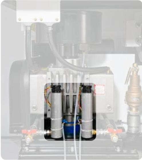
Oil level sensors and oil temp sensors
