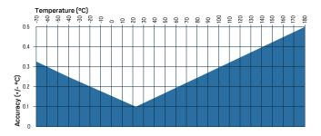
HMP5 temperature measurement accuracy over full range
