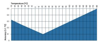
HMP7 temperature measurement accuracy over full range
