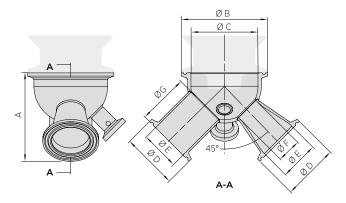
SEFC Sanitary Elbow Flow Cell, reduced inlet
