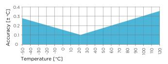
HMP80L temperature measurement accuracy over full range
