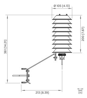
Solar Radiation Shield DTR502B dimensions
