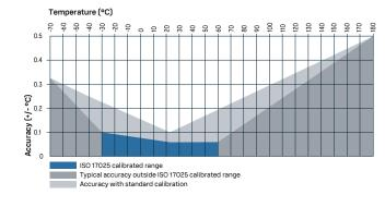
TMP1 temperature measurement accuracy over full range
