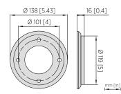
Dimensions of PR53AP tank bottom welding flange
