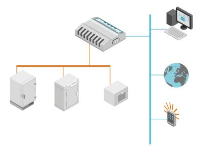
DL1016-1416 data loggers can be used with Vaisala software, either viewLinc or vLog, to download, display, and analyze environmental data.
