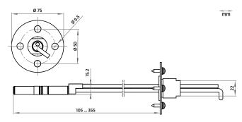
Duct installation kit 210697 dimensions with probe
