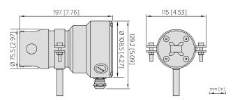
Dimensions of PR53M flow cell end plate bolts (NPT fitting)
