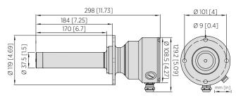
Dimensions of PR53AP tank bottom flange, depth 170 mm
