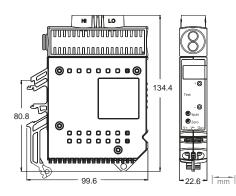
$\ensuremath{\mathsf{PDT102}}$  dimensions with process valve actuator and test jacks
