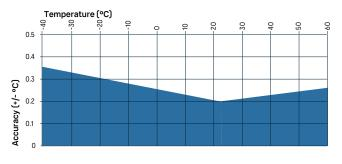
HMP1 temperature measurement accuracy over full range
