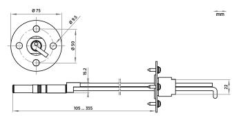
Duct installation kit 210697 dimensions with probe
