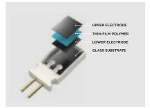
Structure of the HUMICAP sensor
