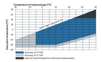
Dew point accuracy vs. measurement conditions
