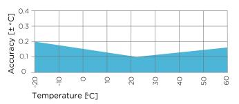
HMP80N temperature measurement accuracy over full range
