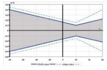
HMP155 accuracy over temperature range: voltage and RS-485
