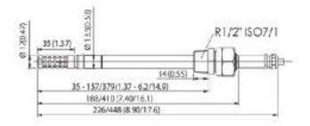
MMT318 probe, dimensions in mm (inches)
