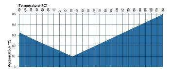
HMP4 temperature measurement accuracy over full range
