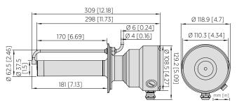
Dimensions of PR53AP Sanitary 4", depth 170 mm, with wash nozzle
