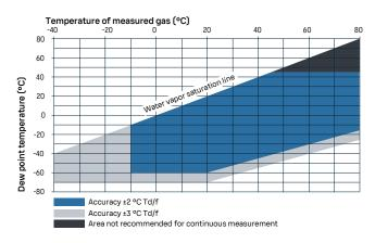
Dew point accuracy vs. measurement conditions
