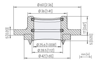
Probe mounting flange 243261SP dimensions, cross section
