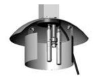
For calibration, a portable HMP77 reference probe is easy to attach beside the HMP7 probe head.
