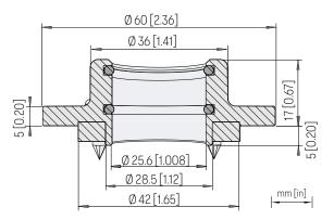
Probe mounting flange 243261SP dimensions, cross section
