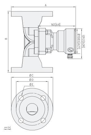
Dimensions of PR53W valve body
