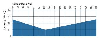
HMP3 temperature measurement accuracy over full range
