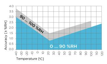
HMP80L humidity measurement accuracy as a function of temperature
