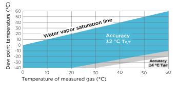
Dew point accuracy vs. measurement conditions (DMP80A)
