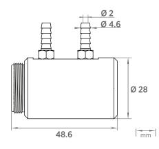
Flow-through adapter with gas ports ASM212011SP. Suitable for tubes with 4 mm inner diameter.
