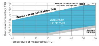
Dew point accuracy vs. measurement conditions (DMP80B)
