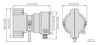
Dimensions of PR53M flow cell end plate bolts (integrated fittings, Flare and Pillar-type)
