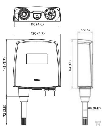
Dimensions of HMP110 remote probe (top image) and HMT120, HMT130, TMT120, and TMT130 transmitters
