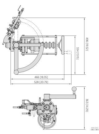
Dimensions of PR53 SDI5 Safe-Drive isolation valve and retractor
