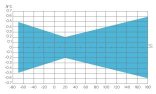
Temperature measurement accuracy over temperature range
