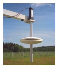
PTB210 paired with SPH10 static pressure head
