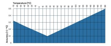
HMP8 temperature measurement accuracy over full range
