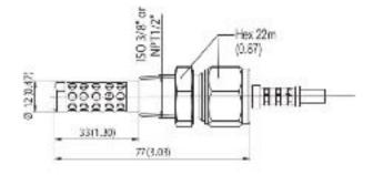
MMT317 probe, dimensions in mm (inches)
