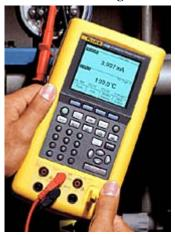
Current and/or voltage simulation of process signals is performed with a simulator that allows entry of the desired current/voltage signal. Simulators are designed for both voltage and current simulation Although any power supply that presents the appropriate voltages could be used for voltage calibration, only a source designed specifically for process signal calibration will allow for suitable adjustment and accuracy to perform calibration.
